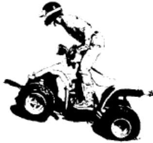
Figure 2. Keep both feet firmly on the footrests and shift your body weight forward when climbing a hill
