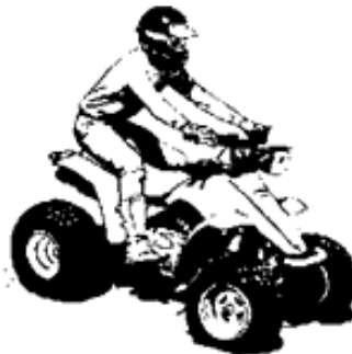
Figure 3. Shift into low gear and point the ATV directly downhill when descending a slope
